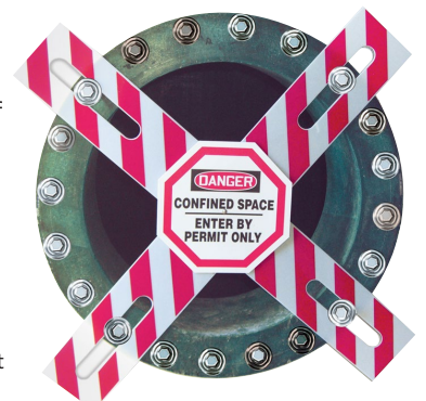
CXB631 Cross Barrier, plastic 1.5" x 11.5" octagonal sign with 5.75" x 42" crossbuck arms Fits 22" to 38" outside bolt-to-bolt
